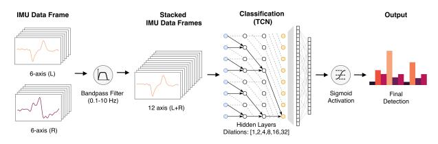
Fig. 4. ExpressEar's processing and classification pipeline overview. Our temporal convolutional network (TCN) architecture comprises several convolutional units (four shown here) and one fully connected layer with sigmoid activation.
