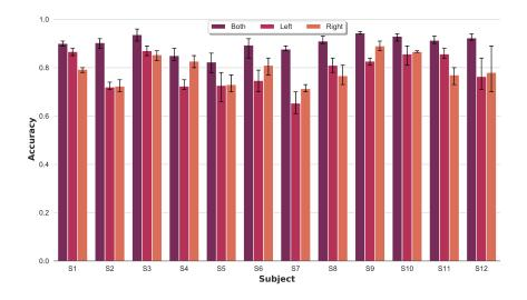
Fig. 7. Per-user Accuracy of all subjects across 3 IMU positions: mounted in left ear, right ear and both ears. The error bar indicates the variation across different folds.
